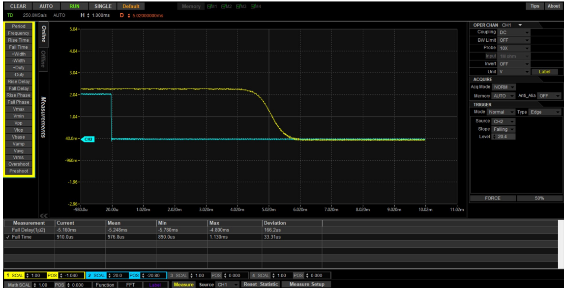
Figure 4.1: Ultrascope software displaying oscilloscope output during mechanical shutter test. The blue line indicates the TTL signal from the function generator. The yellow line indicates optical power measured with a Thorlabs power meter.
